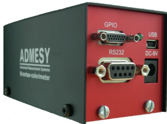
Illustration 1: Brontes colorimeter electrical interfaces.
